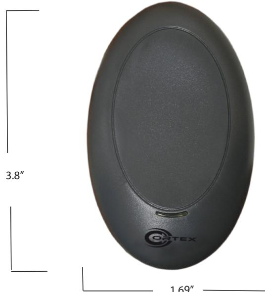
The COR-ACC940 Wiegand proximity card reader is an advanced access control device in a grey ABS case that uses a built-in bicolored LED and beeper to provide users with a visual and audible indication that a card has been scanned. It can operate in standalone mode or in networking configurations. Built-in watchdog function prevents system lock-up. Sealed for outdoor use. Attached cable and plug connector make installation simple.
