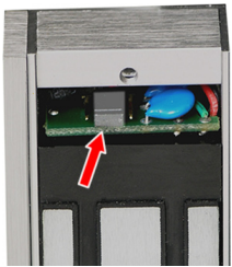
Jumper Setting for 24VDC Operation
