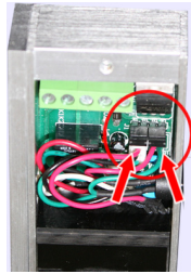
Jumper Setting for 12VDC Operation (Default Setting)
