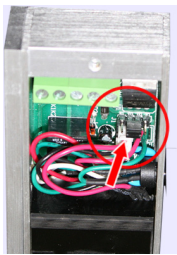
Jumper Setting for 24VDC Operation
